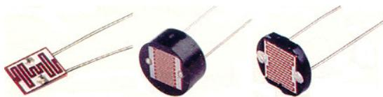
Still another way of counting is by interrupting a beam of light. A component that is of good use for this is the LDR (Light Dependent Resistor). The resistance of an LDR becomes lower when it catches light. With an Ohm meter you can measure the value at the light intensity that you
